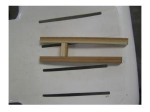
5. It is now time to prepare the track support DECK (between track and the bents). My selection for both straight and curved deck is 3/4 by 3/4 red wood longerons, spaced 1-1/2 in apart with 3/4 by 3/4 blocks every 9 inches.
